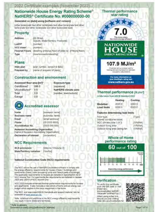
Figure 13-4: NatHERS Certificate Whole of Home produced by an Accredited Assessor (right) for NCC 2022
