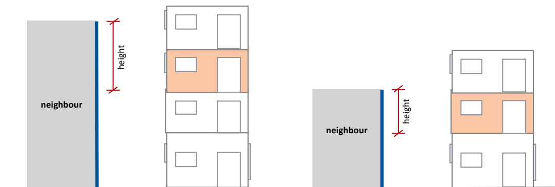
Figure 10-12: Elevations of vertical shading height for Class 2 dwellings*
