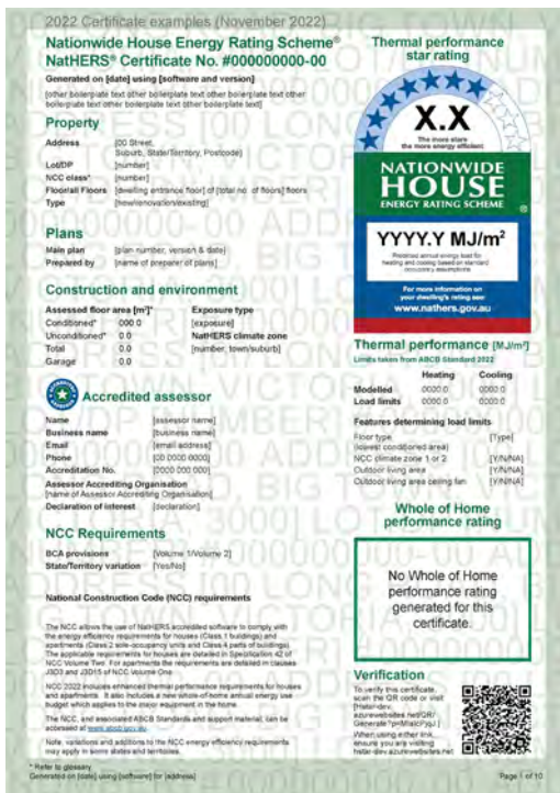
Figure 13-3: NatHERS Certificate thermal only produced by an Accredited Assessor (left) for NCC 2022
